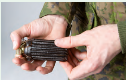
The lever part is in the hand you throw with while the other hand twists and attaches the body to the lever.
