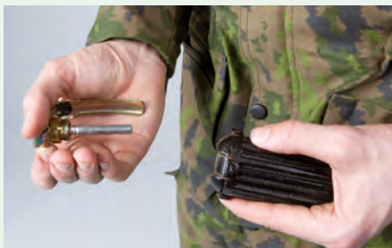
Join the body and the fuse in front of your body.
