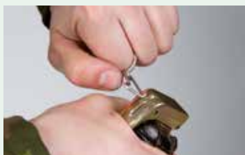
Pull the safety pin from fuse with a straight pull after which the hand grenade is ready to be thrown.
